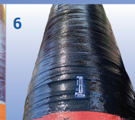
6 Coating protection and smart traceability tag
