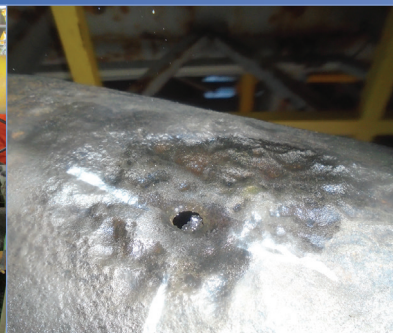
THROUGH WALL DEFECT, LEAK, HOLE
