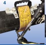
Tighten until leak is sealed 40 N.m (354 in-lb) max.
